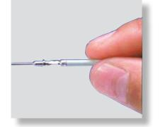
1. Grasp crimped contact approximately 1.0" (25.4mm) behind the contact barrel.
