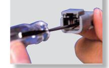
2. To remove the contacts, gently pull wire backwards, while at the same time releasing the locking finger by moving it away from the contact with a screwdriver.
