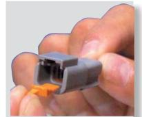
4. Once all contacts are in place, insert orange wedge: receptacles - with half holes aligning with contacts. Plugs - with contacts aligning behind full holes. The orange wedge will snap into place.
