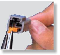
1. Remove orange wedge using needlenose pliers to pull wedge straight out.
